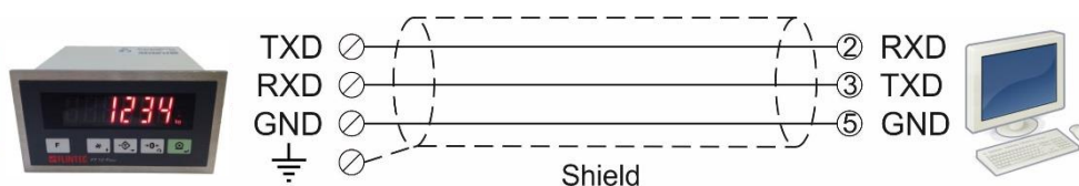
Figure 4.3 - RS 232C serial interface connections
